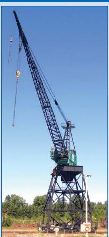
**COLBY** Mobile Gantry Crane, Model 240, 45 Ton Capacity, Radius Range 67' - 143', Up To 30 FPM, Plus 5 Ton Auxiliary Hoist at Any Radius, Up To 150 FPM, Cab Operated Full Control, Crane Smart Digital Readout, Hoist Room Monitor, Gantry Bridge Travel 110 FPM, Travels on Rail, Approx Max Wheel Load at Gantry 80,000 lb, Approx Crane Weight 250,000 lb, 550 V, sn 42121-45-MON-240
