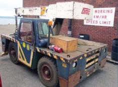
**BMC** Model IC80 1B Mobile Crane, Max 17,000 lb on Outriggers, Max 30', Up To 70 Degree, Cab, sn 813B
