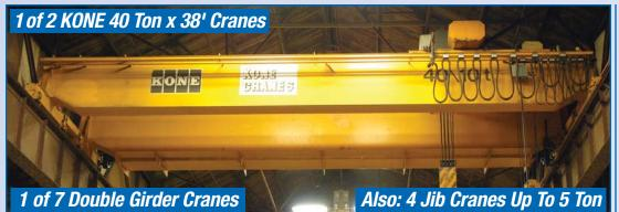
KONE 40/10 Ton Capacity, 38' 1/2" Span
